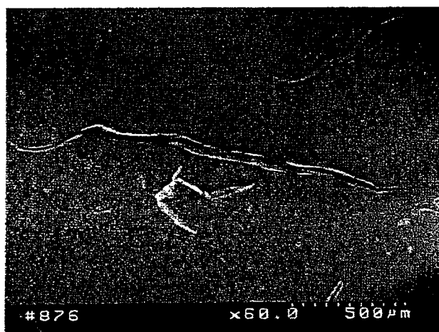
FIGURE 5. Textured McGhan saline implant deflated after 5.5 years in vivo. The SEM micrograph shows 1.5-mm-long tear near outer perimeter, but no evidence of surrounding surface abrasion. Micrograph taken of smooth inner surface of shell exposed to saline.
